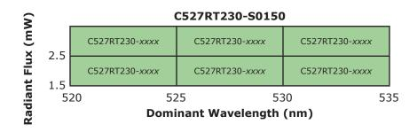
**Note** – Dominant Wavelength shifts shorter with increased forward current ( $I_r$ ). For reference only, the typical DW shift from 5 to 20 mA is -2 nm for Blue LEDs (4xx nm) and -7 nm for Green LEDs (5xx nm).
