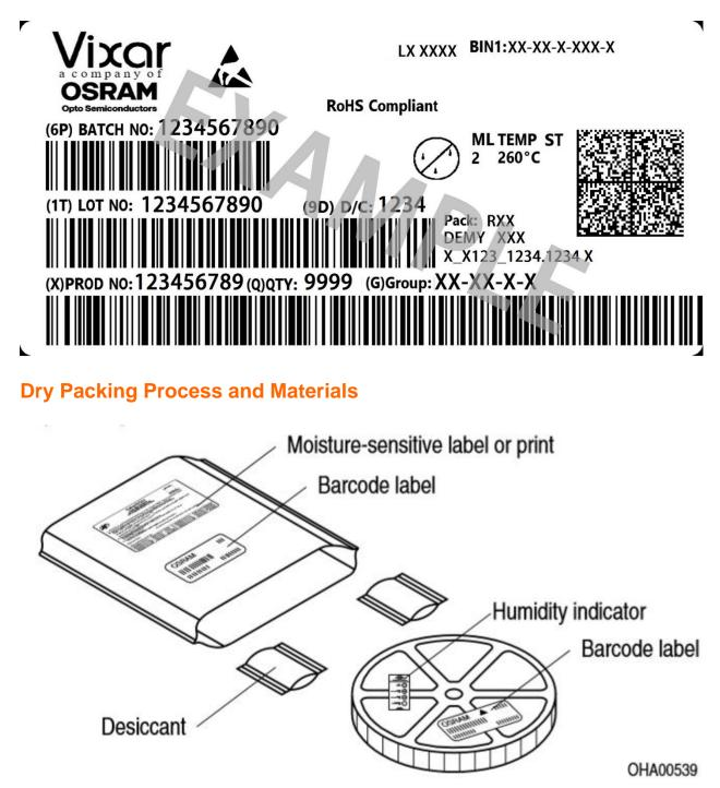
Moisture-sensitive product is packed in a dry bag containing desiccant and a humidity card according JEDEC-STD-033.
